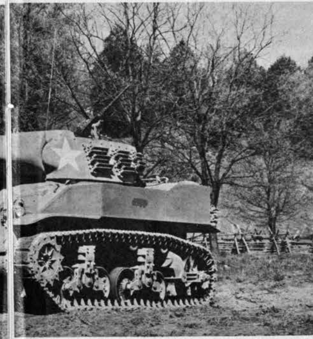
large trailing idler in direct contact with the ground promotes speed at the expense of durability and is characteristic of all three of the armored vehicles on this page.
